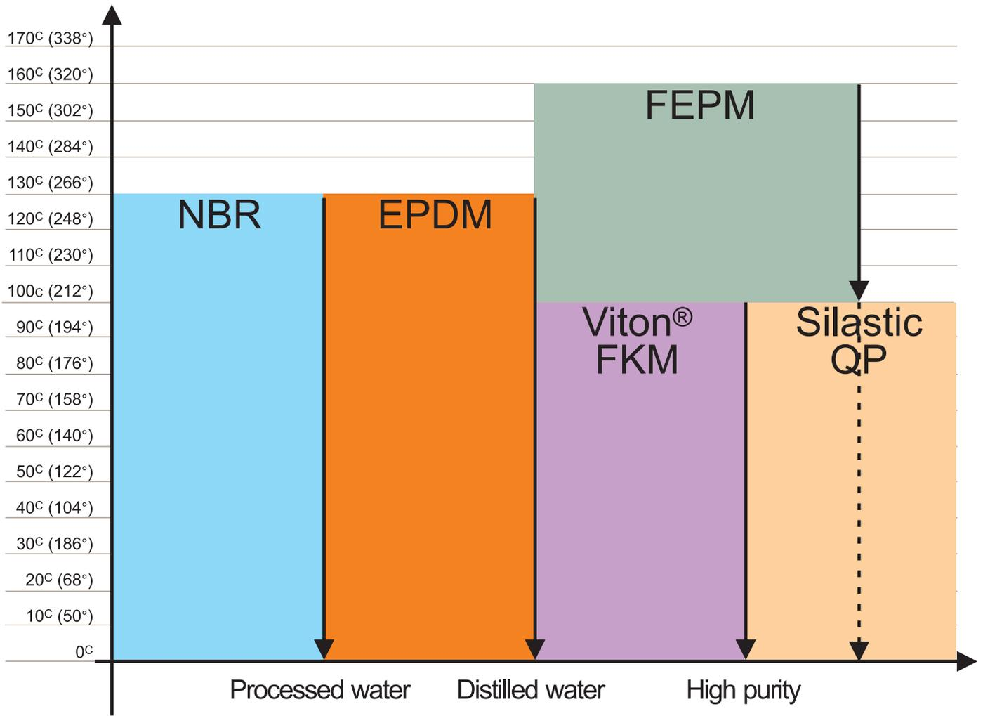
Alfa Laval can provide additional technical gasket material information. Contact your Alfa Laval thermal specialist for details and technical specifications as it relates to your operating requirements.
